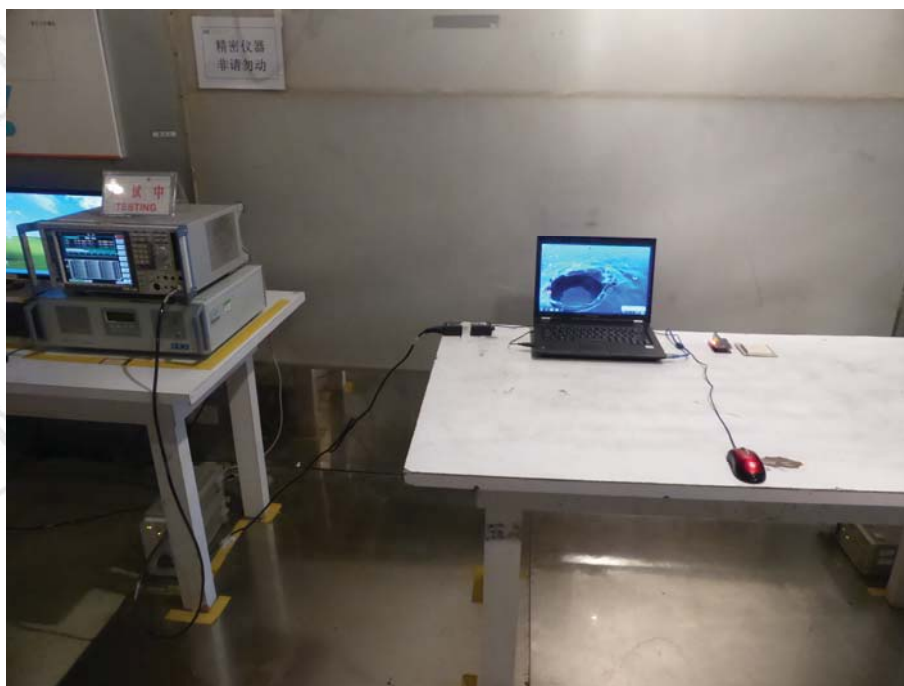
TEST SETUP OF CONDUCTED EMISSION
