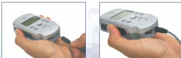
Figure 12. Switching on the GSM Controller
