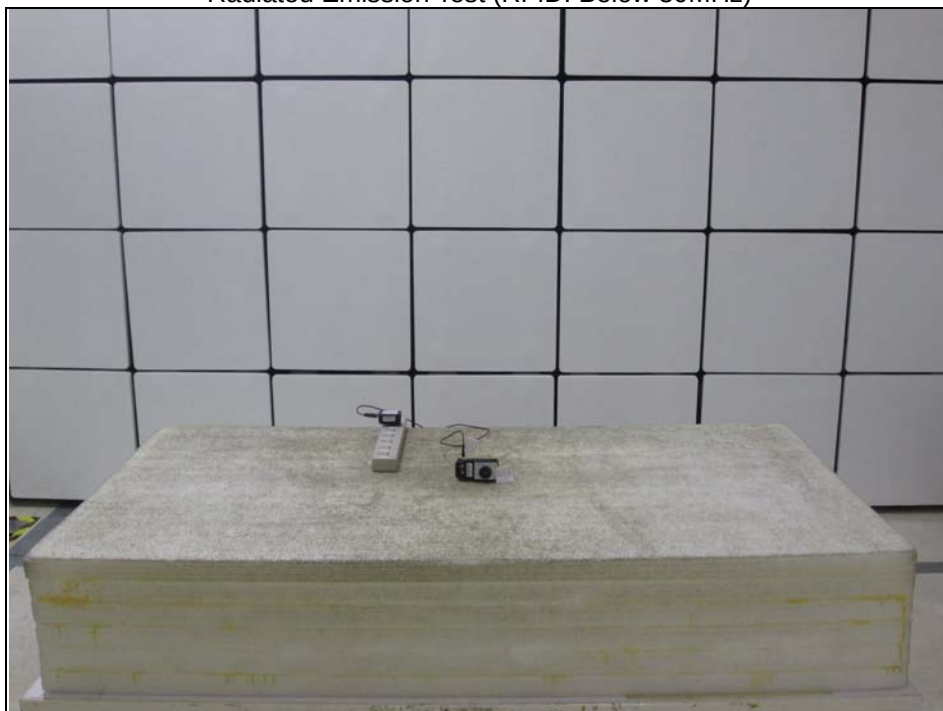
Radiated Emission Test (RFID: Below 30MHz)
