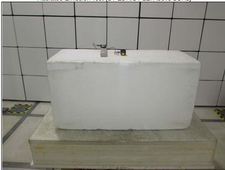
Radiated Emission Test (BT EDR/BT LE: Above 1GHz)
