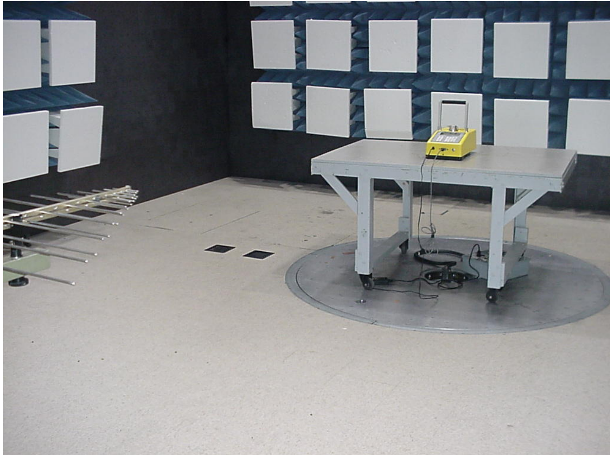
Figure 5 - Radiated Emissions Test Setup (Chamber - Front)
