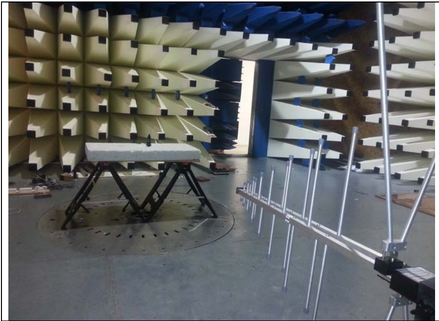
Fig 1 Test setup 30MHz -300MHz Rad Emissions
