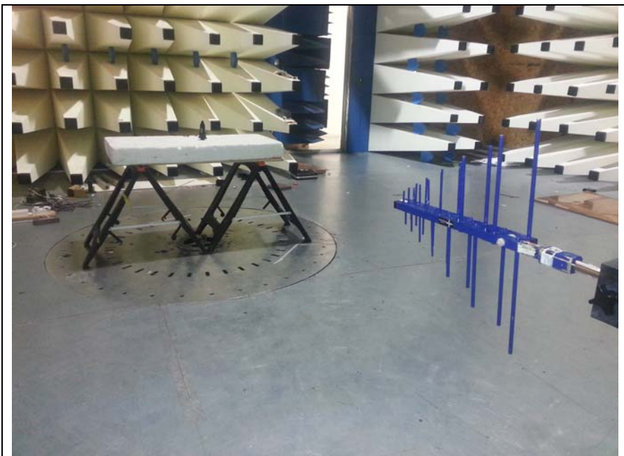
Fig 2 Test setup 300MHz -1GHz Rad Emissions
