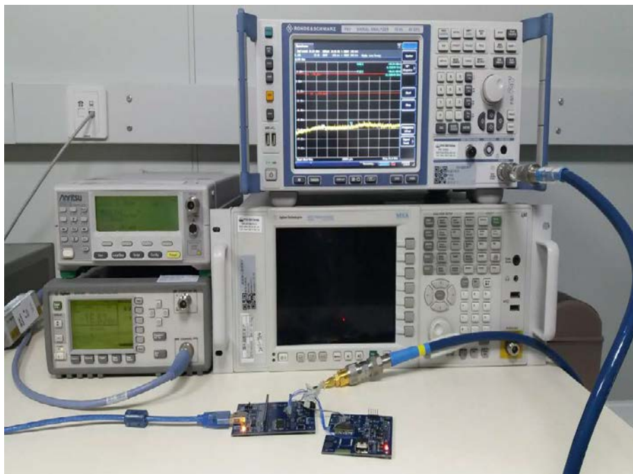
Spurious RF Conducted Emissions Test setup
