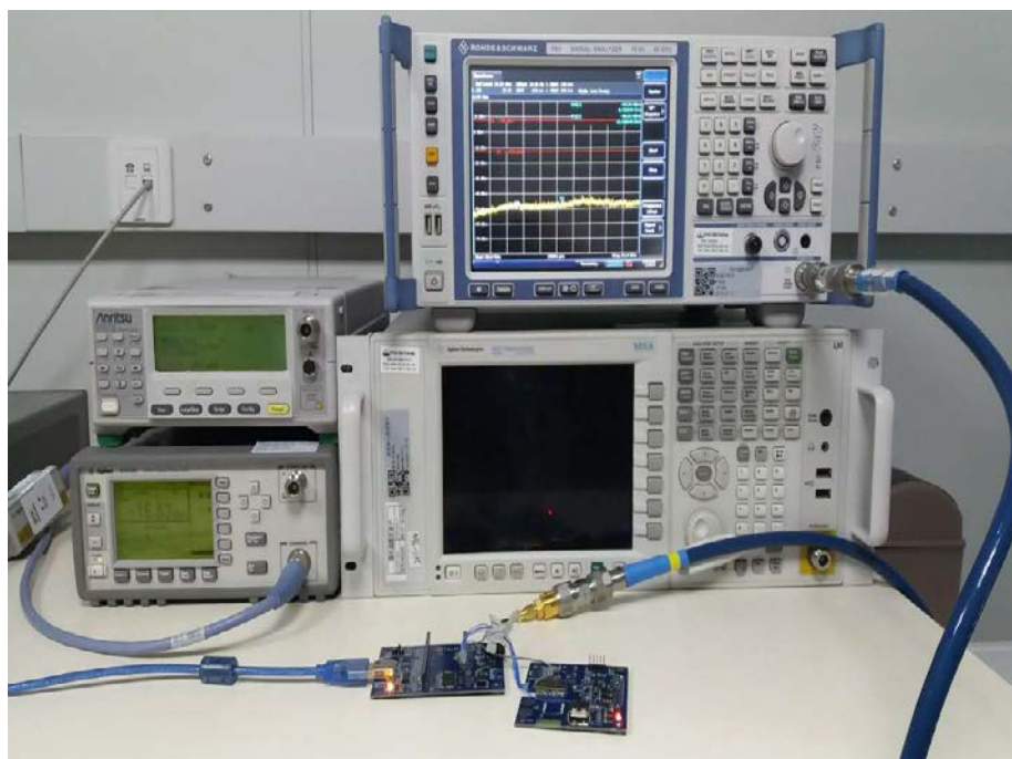
Spurious RF Conducted Emissions Test setup
