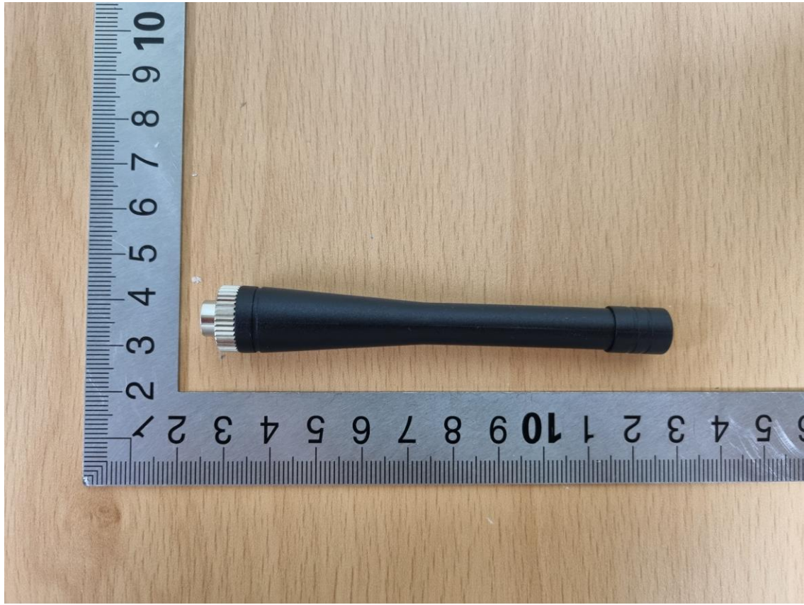
Dipole Antenna (WE11-BO-21 _ 3.0 dBi)
