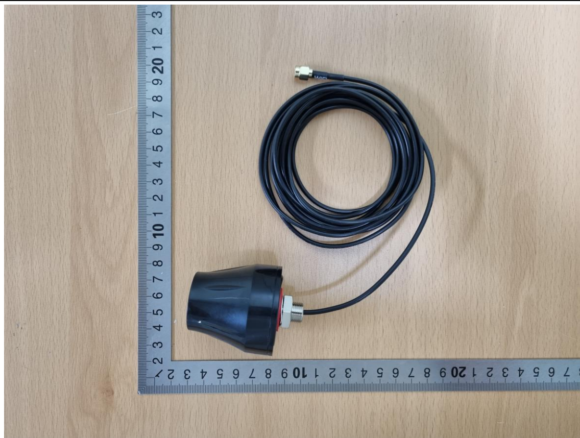
Dome Antenna (WBZ28 _ 0.0 dBi)
