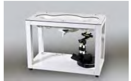
Figure 3.5.1 SAM Twin Phantom
