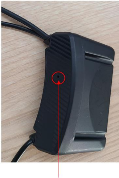
Pinhole Fault Reset Button
