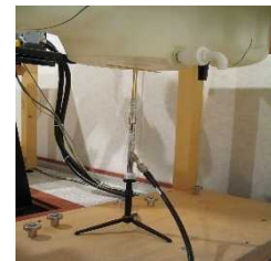
Photo of the dipole Antenna
