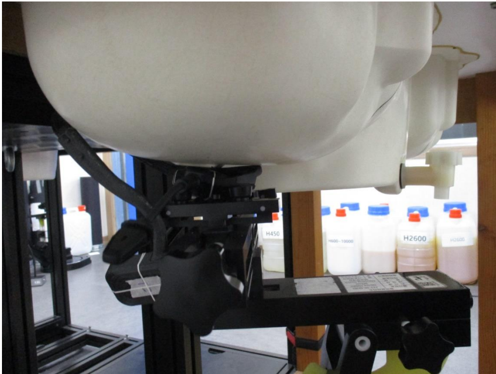
Right Ear from SAM Phantom (Separation Distance: 0 cm) – MESH Antenna.1
