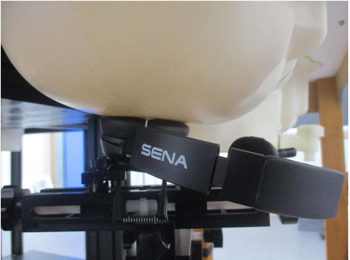
Right Ear from Head Phantom (Separation Distance: 0 cm)
