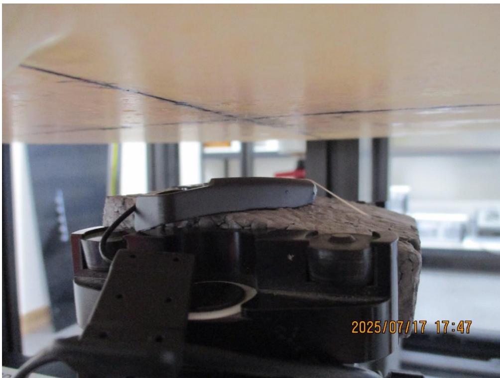
Rear Side from Flat Phantom (Separation Distance: 2 cm)
