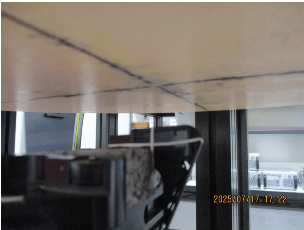
Left Side from SAM(Flat) Phantom (Separation Distance: 2 cm)
