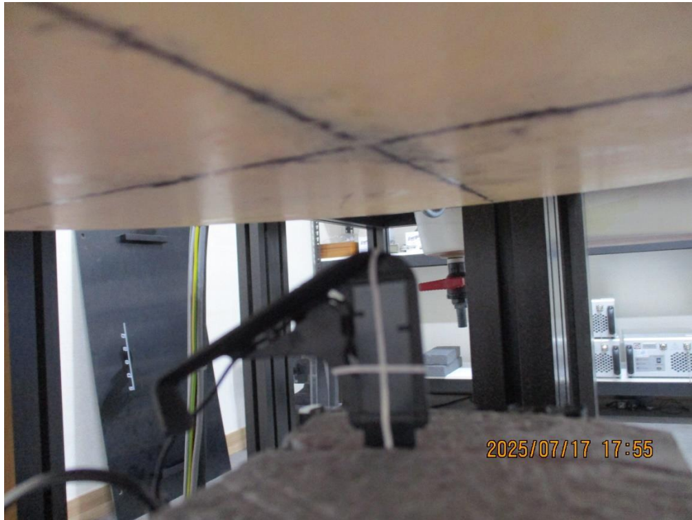
Top Side from Flat Phantom (Separation Distance: 2 cm)
