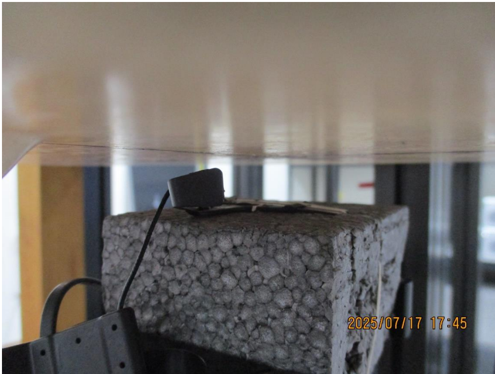
Front Side from Flat Phantom (Separation Distance: 2 cm)
