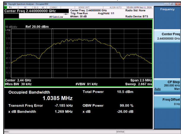
BLE 1M Mid Channel – Occupied Bandwidth
