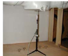
Figure 9.1 Dipole Verification Test Setup Diagram & Photo
