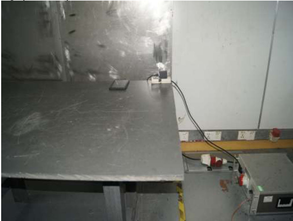
Photograph 2: Set-up for Spurious Emissions for below 30MHz
