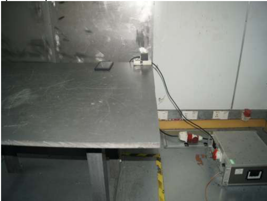
Photograph 2: Set-up for Radiated Emission of below 1GHz
