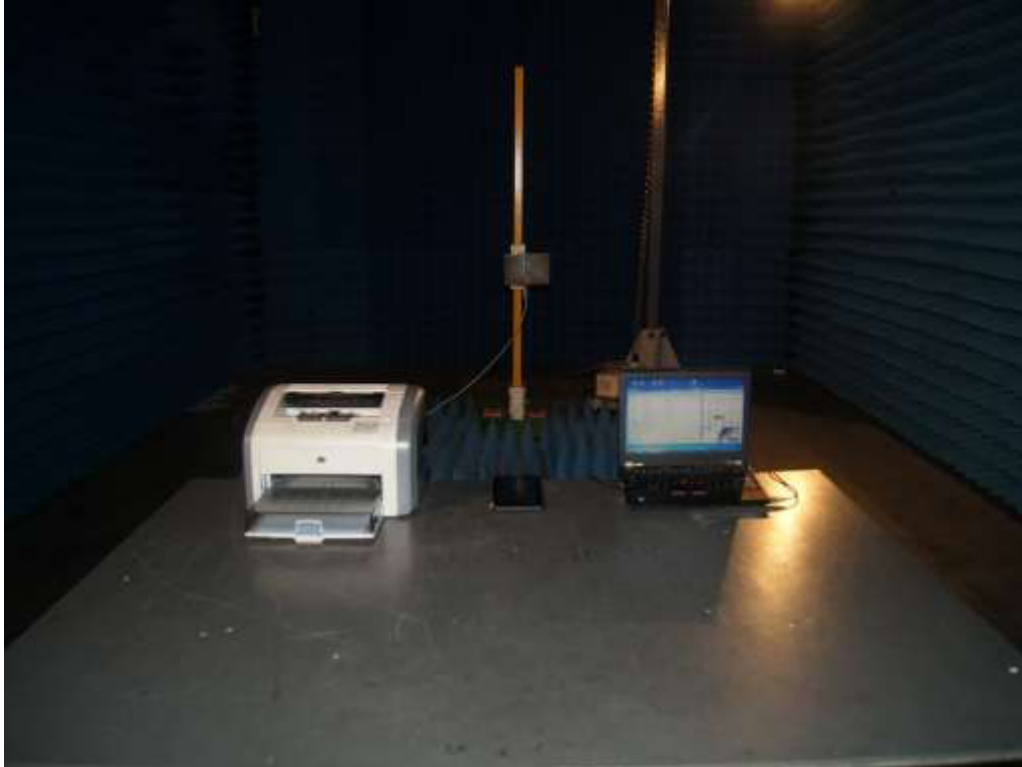
Photograph 4: Set-up for Radiated Emission of 18 - 25GHz
