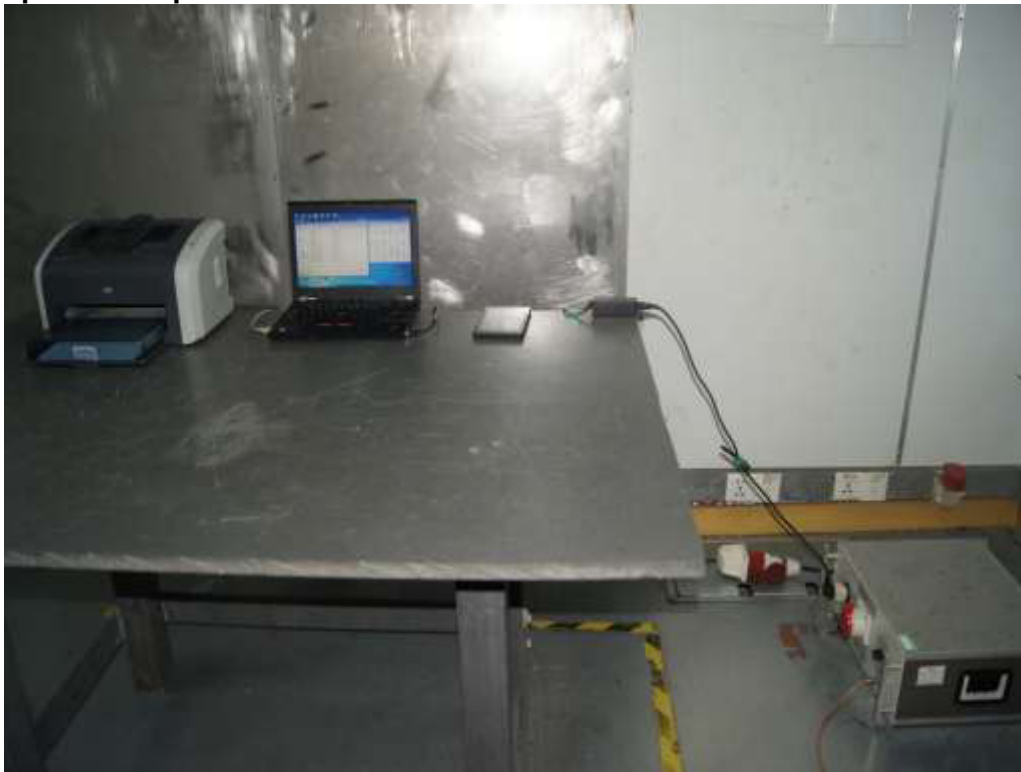
Photograph 2: Set-up for Radiated Emission of below 1GHz
