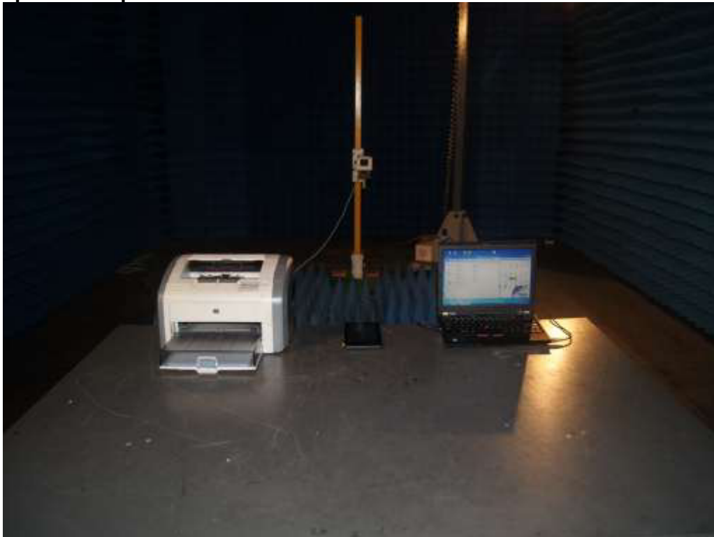
Photograph 4: Set-up for Radiated Emission of 18 - 25GHz
