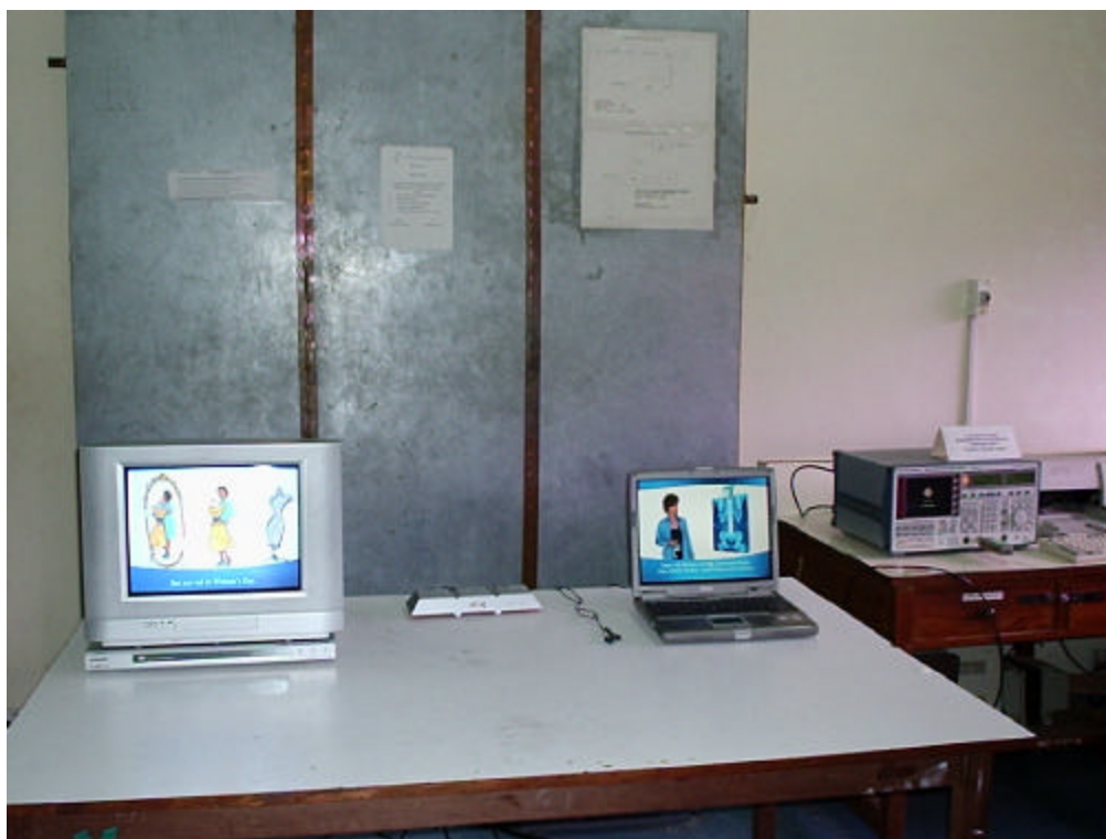
Photograph 1: Set-up for Conducted Emission on AC Mains
