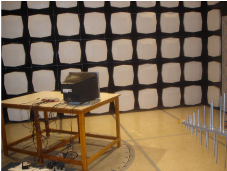
Photograph 2: Set-up for Radiated Emission in Vertical Orientation
