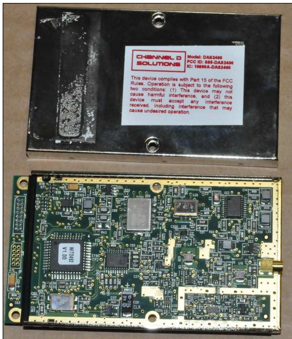
Figure 5: Internal Photo – RF Module installed with Bottom Shield, Top Shield Removed
