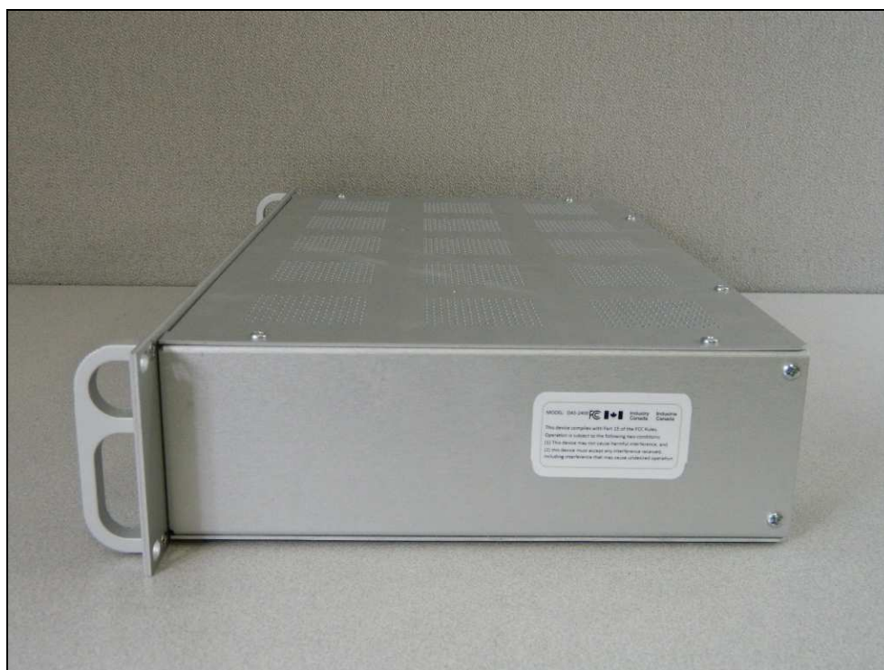
Figure 2: Sample Label Location - DAS2400 antenna distribution chassis
