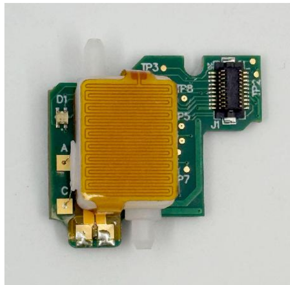
Alcohol Sensor PCBA, with sensor. Front view with slight angle to show PCBA.
