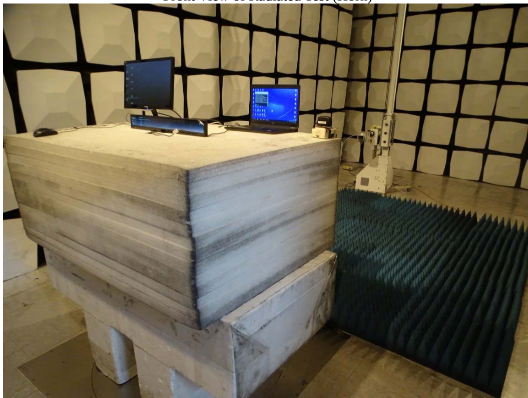
Front View of Radiated Test (Horn)
