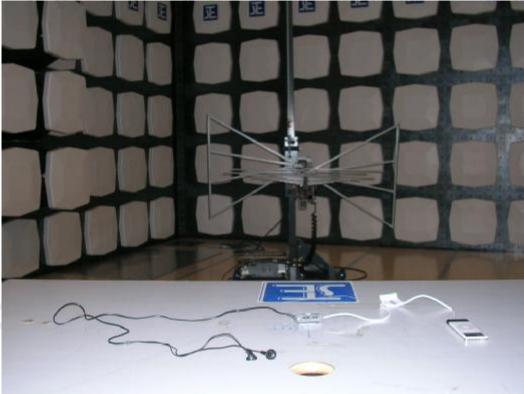
Measurement of Radiated Emission Test Set Up
