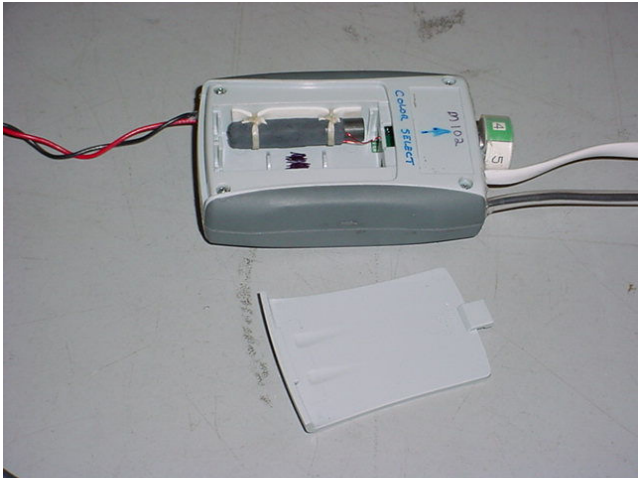
M Unit, Battery Compartment and RFID Antenna. Rear Cover Removed.
