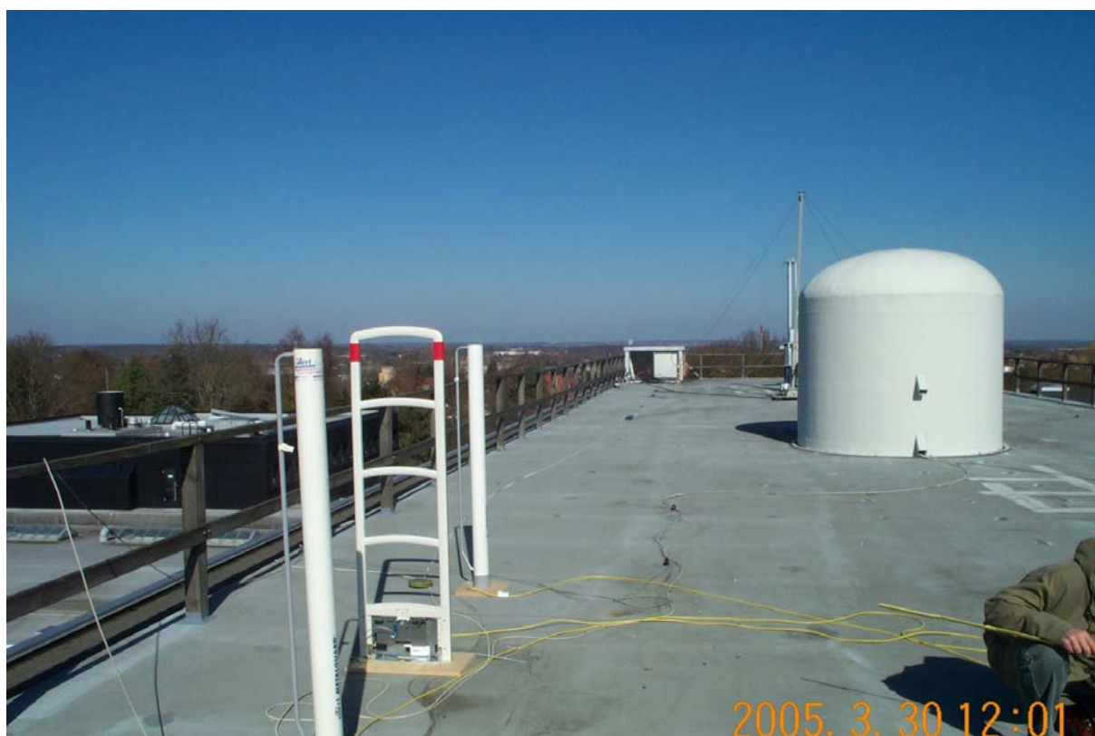
Photo 4 Radiated emission. 30 m OATS.
