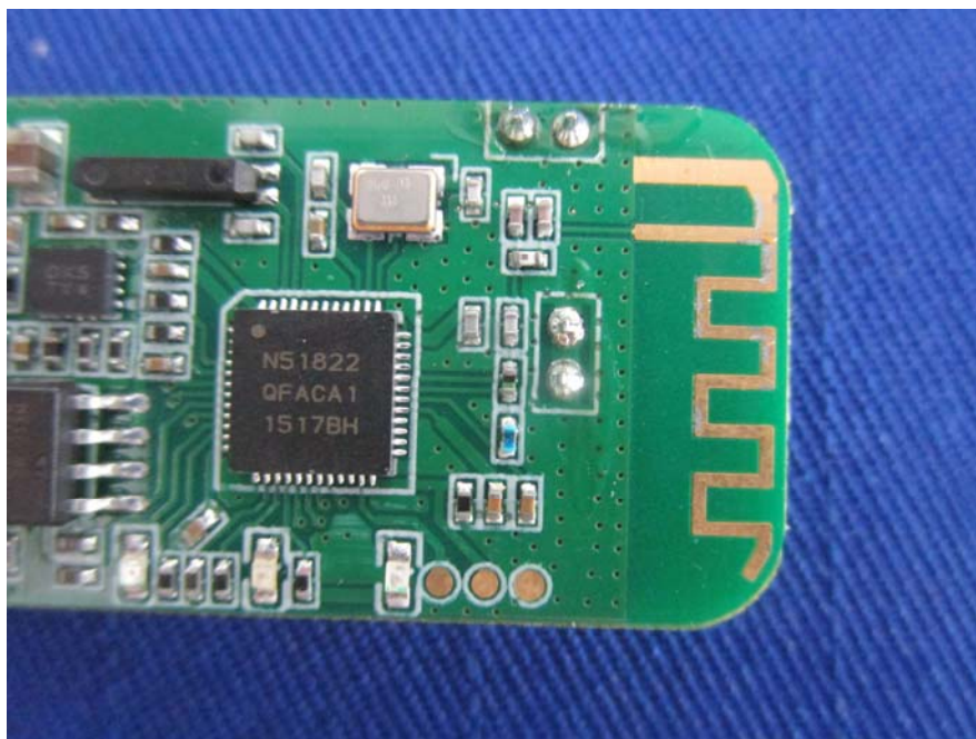
EUT –Antenna & RF Chip View
