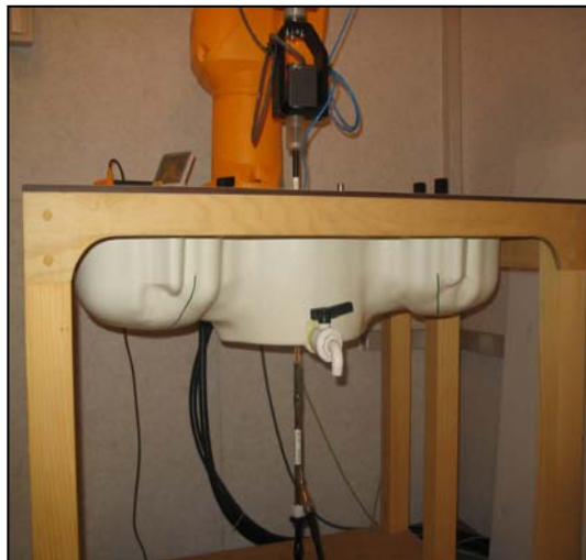
< Photo 4. 2450 MHz Validation Setup >
