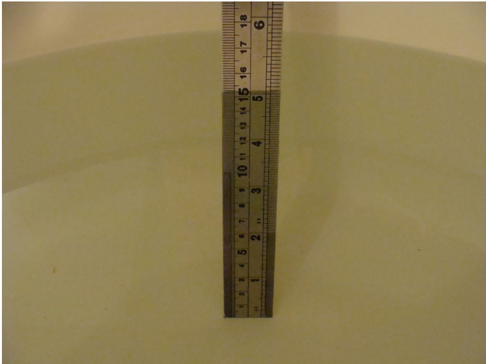
Depth of the liquid in the phantom
