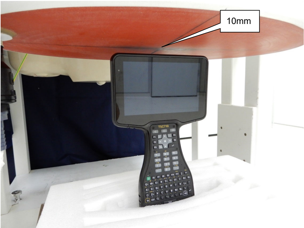
EUT Top -10mm (Main Antenna)
