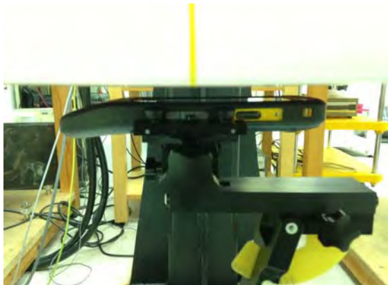
Fig.7 EUT front to flat phantom
