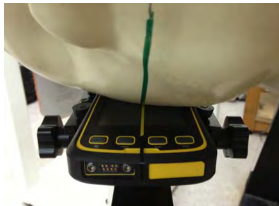
Fig.3 Right Head Section / Cheek-Touch Position
