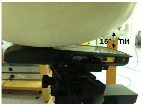
Fig.4 Right Head Section / Ear-Tilt Position(15°)
