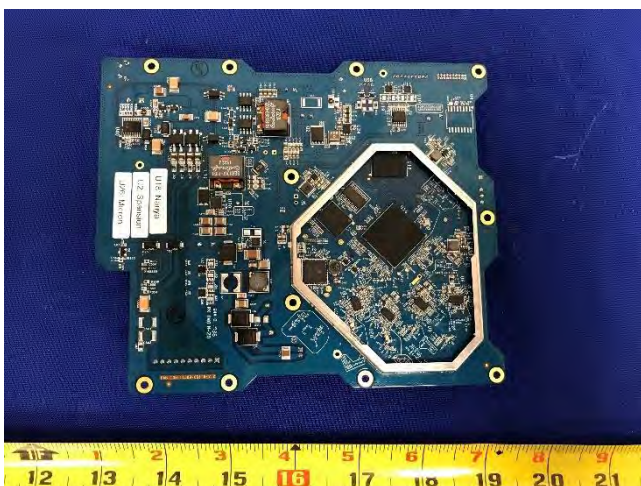
Modem Board Bottom View without shielding
