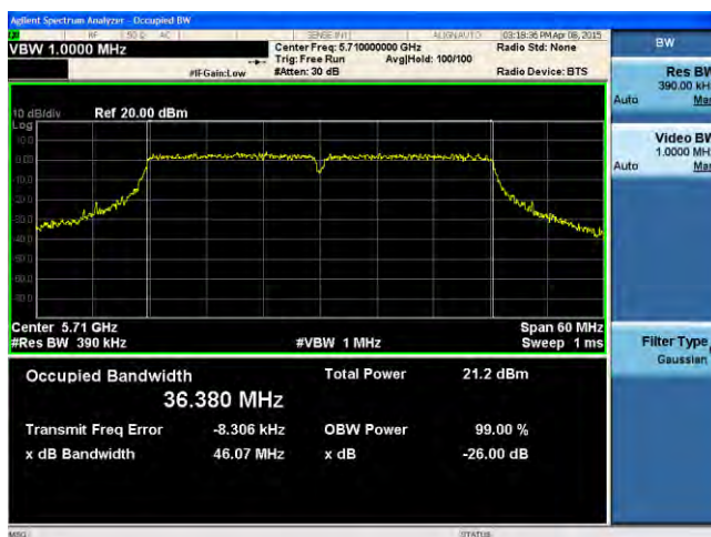
26dB BW -802.11n-HT40-CROSS BAND-5710MHz
