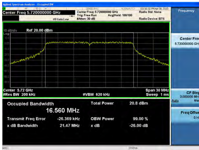
26dB BW -802.11a CROSS BAND-5720MHz
