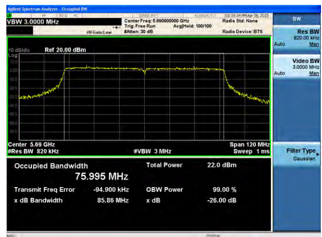
26dB BW -802.11ac-CROSS BAND-5690MHz
