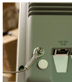
FIGURE 5 Attaching Security Cable to AP
