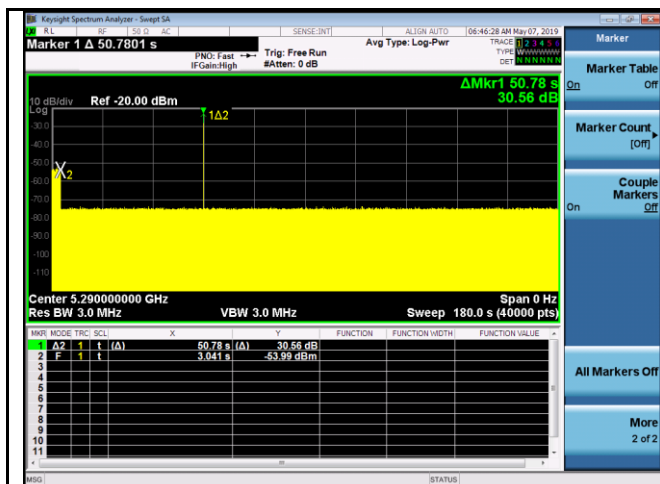
Radar at beginning of CAC – 802.11ax-80 – 5290MHz
