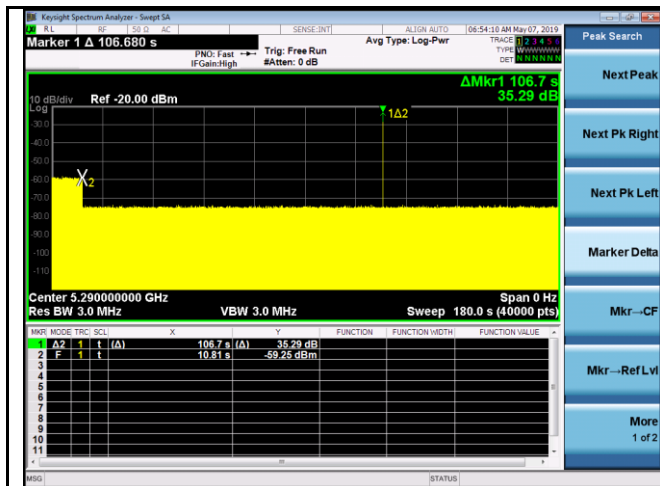
Radar at end of CAC – 802.11ax-80 – 5290MHz
