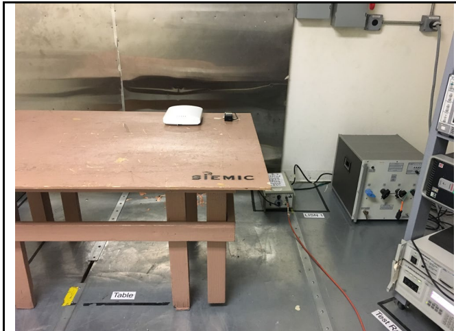
Conducted Emission – Front View
