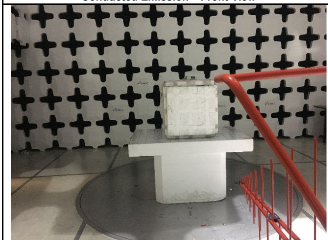
Radiated Emission Below 1G – Front View
