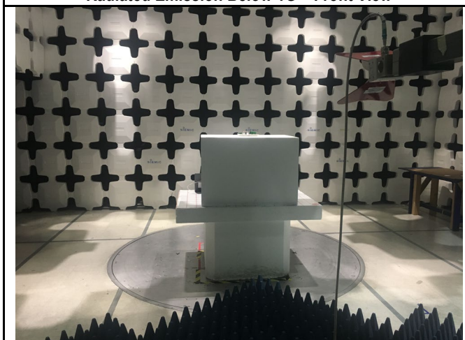
Radiated Emission Above 1G – Front View
