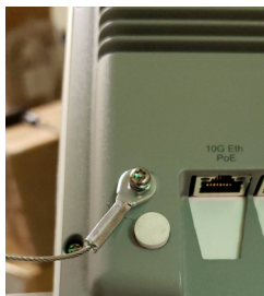
FIGURE 5 Attaching Security Cable to AP
