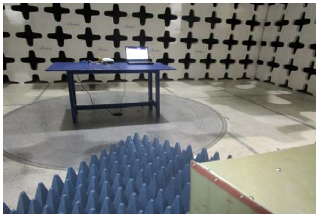
Radiated Emissions (>1GHz) – Front View
