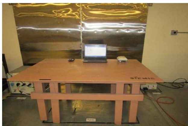
Conducted Emissions - Power Supply Mode – Front View
