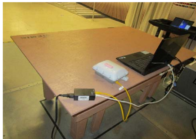
Conducted Emissions - P.O.E Mode – Rear View
