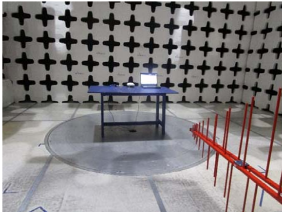
Radiated Emissions (<1GHz) – Front View
