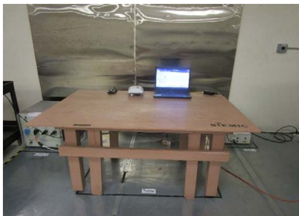
Conducted Emissions - P.O.E Mode – Front View
