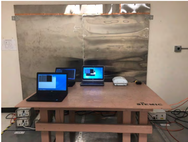
Conducted Emissions - Power Supply Mode – Front View
