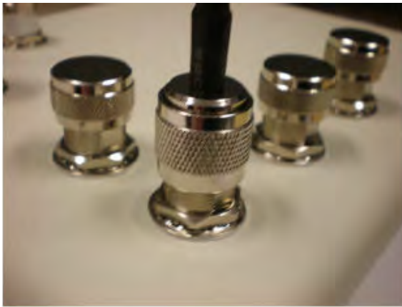
FIGURE 12 Connecting the Cable with the Connector
