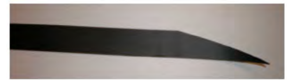
FIGURE 16 Cutting the Sealing Tape at an Angle
