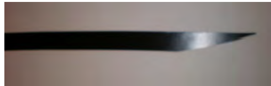
FIGURE 14 Cutting the End of the Electrical Tape
