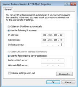
Figure 8. Sample configuration in the Internet Protocol Version 4 (TCP/IPv4) Properties dialog
