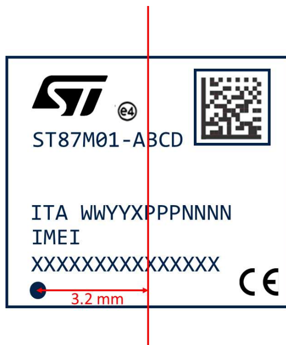
Figure 18: Module Marking Information (RED)
