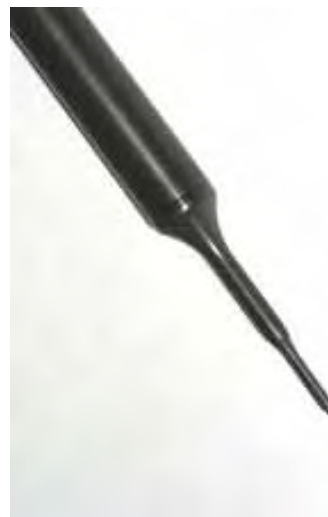
Fig. 5.2 EX3DV4 E-field Probe
