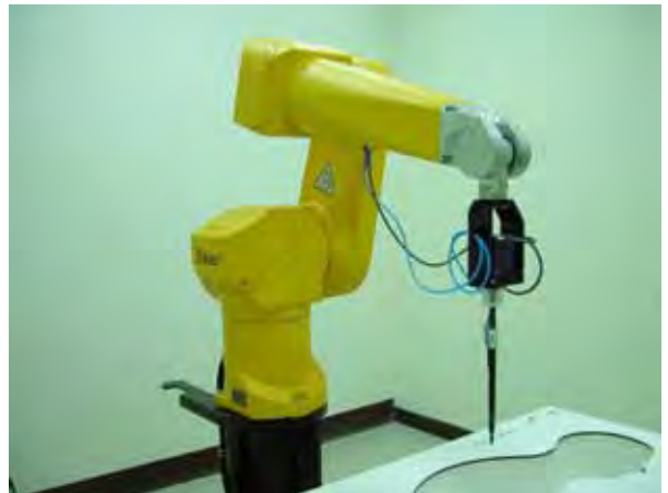
Fig. 5.2 Probe setup on robot
