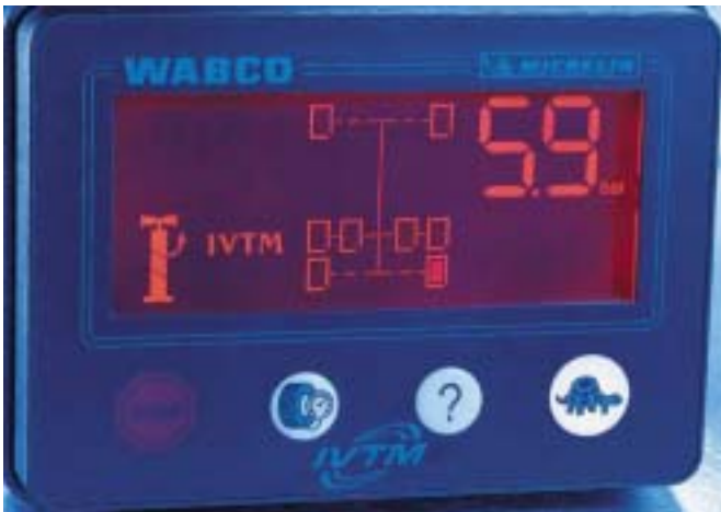
red indicator light button button yellow indicator light STOP Manometer symbol „?“ Turtle symbol
