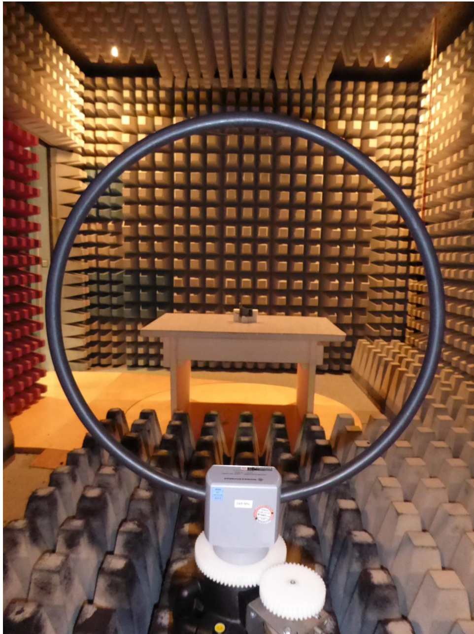
162386_20.JPG: WM2.4, test set-up fully anechoic chamber
