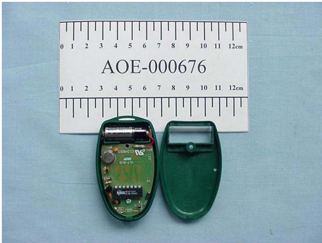
FIGURE 1 REMOTE CONTROLLER (M/N: YLT-5C) COVER REMOVED
