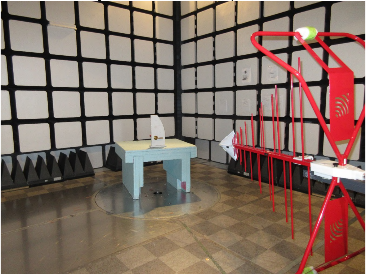
Figure 2 – Radiated Emissions Setup – Photo 2
