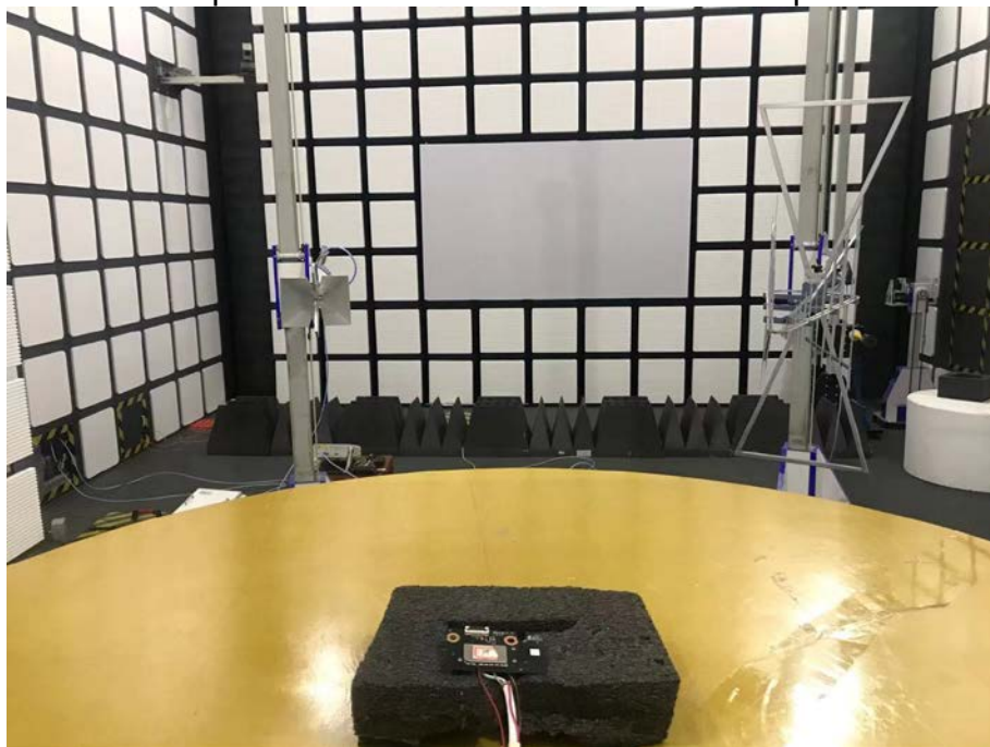
Spurious Radiated Emissions Test setup
