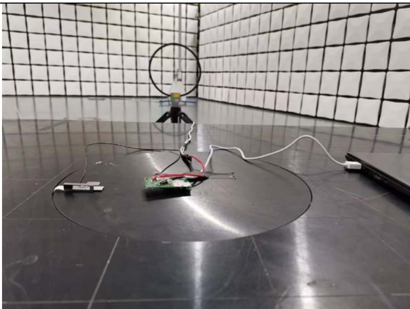
Spurious Radiated Emissions Test setup
